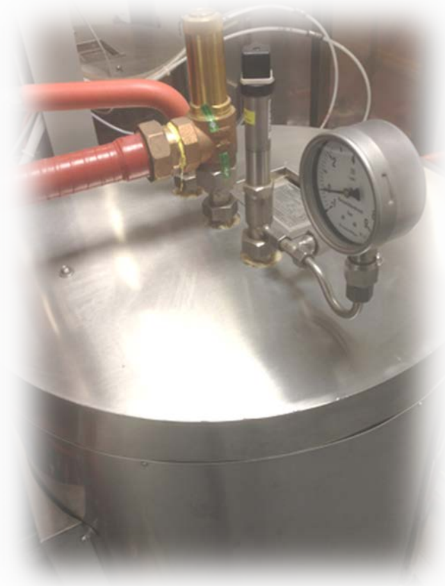
Steam for test purpose according to DIN EN ISO 11140-4: appendix J
