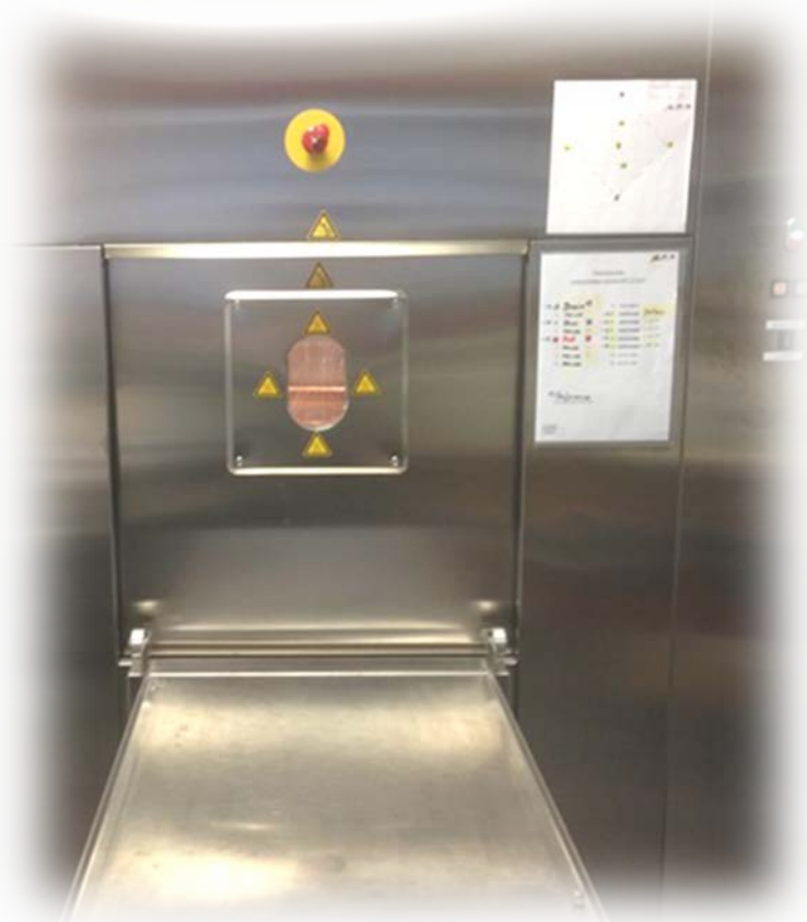
Test steriliser according to DIN EN ISO 11140-4: appendix J
